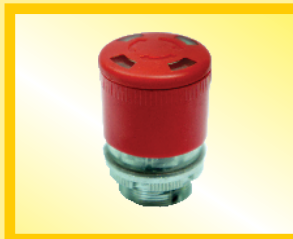
MUSHROOM OPERATOR Ø 30 TURN TO RELEASE EN 418
